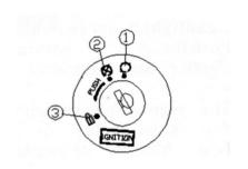
(3) position Turn the switch all the way to the left, push it down and turn to the position; the key can be pulled out. In this case, the vehicle can not be steered and the engine as well as the lighting system will not work.
