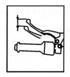
Required free play: 5 to 10 mm. This must be checked with steering at left, right and centre.
