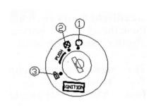
(3) position Turn the switch all the way to the left, push it down and turn to the position; the key can be pulled out. In this case, the vehicle can not be steered and the engine as well as the lighting system will not work.
