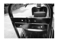
10. Install back the rear backrest on the bottom bracket with the two screws.
