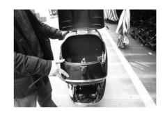
12. Put the longer bolt and the washer through the hole in the rear of the top box highlighted in the photo with the white circle.
