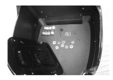
2. Take off the two screws that fixed the rear backrest with screwdriver.
