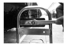
5. Put the iron bottom board centrally on the rear rack.
