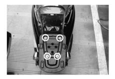
7. Place the four curved brackets underneath the rear rack covering the bars of the rack.
