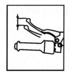
Required free play: 5 to 10 mm. This must be checked with steering at left, right and centre.
