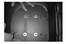
5. Insert the bolts through the four aligned holes in the bottom-board (highlighted in white circles in figure 2). Hold the long slotted bars under the rack with the edges of the bars facing upwards. Put the bolts through the holes of the slotted bars.
