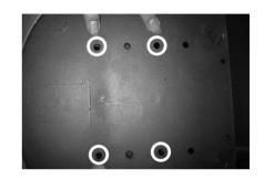
4. With these four holes (highlighted in white circles in figure 3) insert the 4 bolts and 4 washers.
