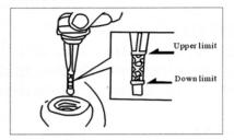
The engine oil dipstick and cap are combined and is located on the right side of the engine. With the bike on its centre stand and on level ground remove the dipstick and clean it. Re-insert it and remove it again. The oil level should be visible on the hatched marking between the lower and upper level. Add or remove as appropriate.
