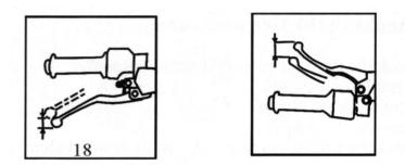
Required free play : 5 to 10 mm. This must be checked with steering at left, right and centre.
